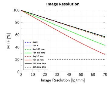
Modulation Transfer Function (MTF) vs. Image Resolution, wavelength range 486 nm - 656 nm from the centre to to the corner of the image at wf/1.4 - close
